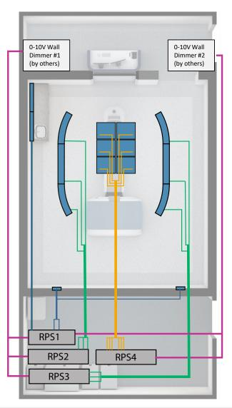
a pre-installed cable connects each luminaire to its respective RPS: 0-10V connection: cables outside of shielded room
